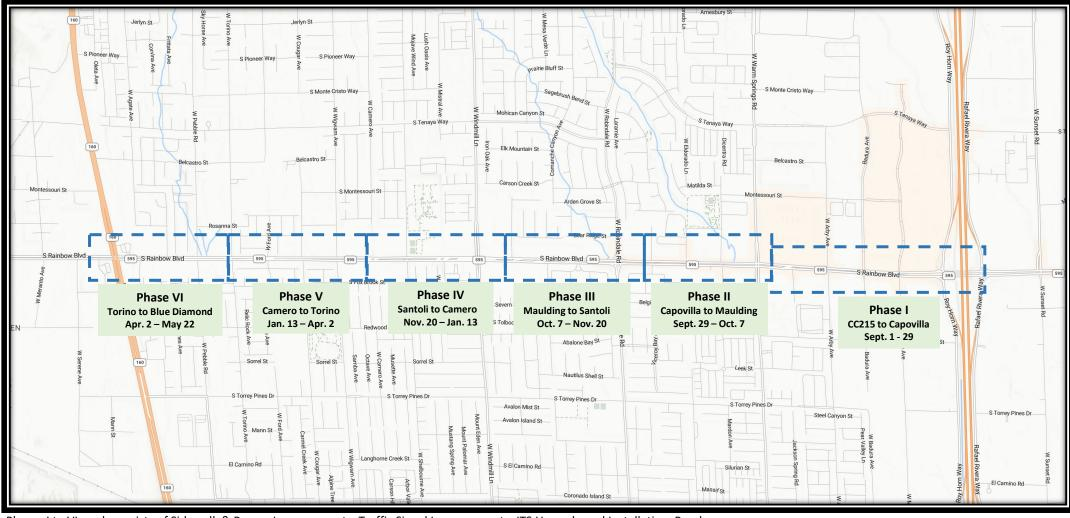
Phases I to VI work consists of Sidewalk & Ramps Improvements, Traffic Signal Improvements, ITS Upgrade and Installation, Roadway Reconstruction, Median Construction, Storm Drain Improvements, LED Luminaire Upgrades, Striping, Signage, and Ultra Thin Asphaltic Concrete Surface.
