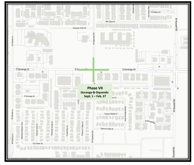
Phase VII work consists of a new Traffic Signal System, Removal of Existing Flasher, ADA Compliant Ramp Installation, Median Construction, Striping and Signage.
