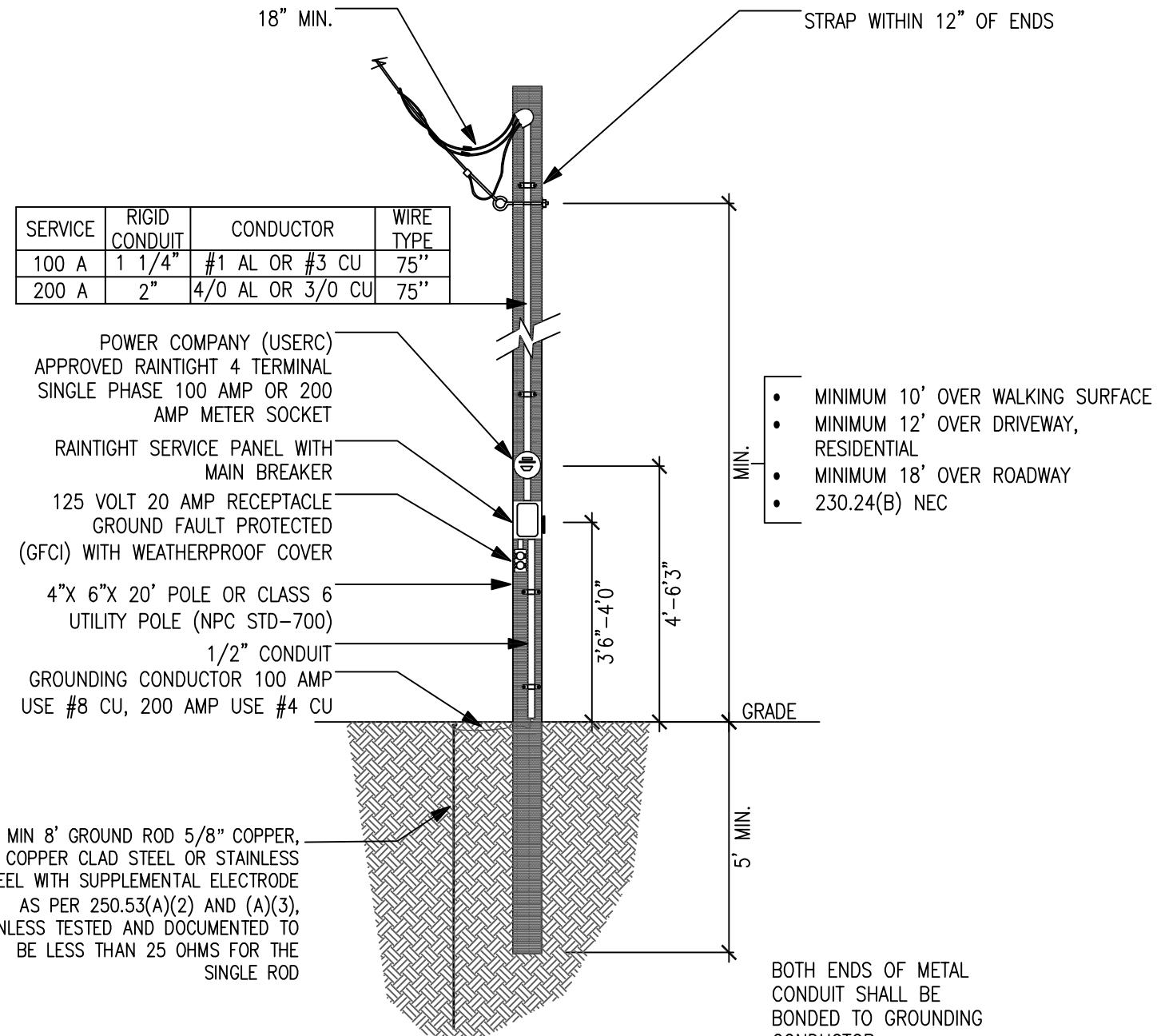
NOTE: WHERE 277/480v POWER IS BEING DISTRIBUTED, THE INSTALLATION MUST COMPLY WITH 590.8B NEC.
