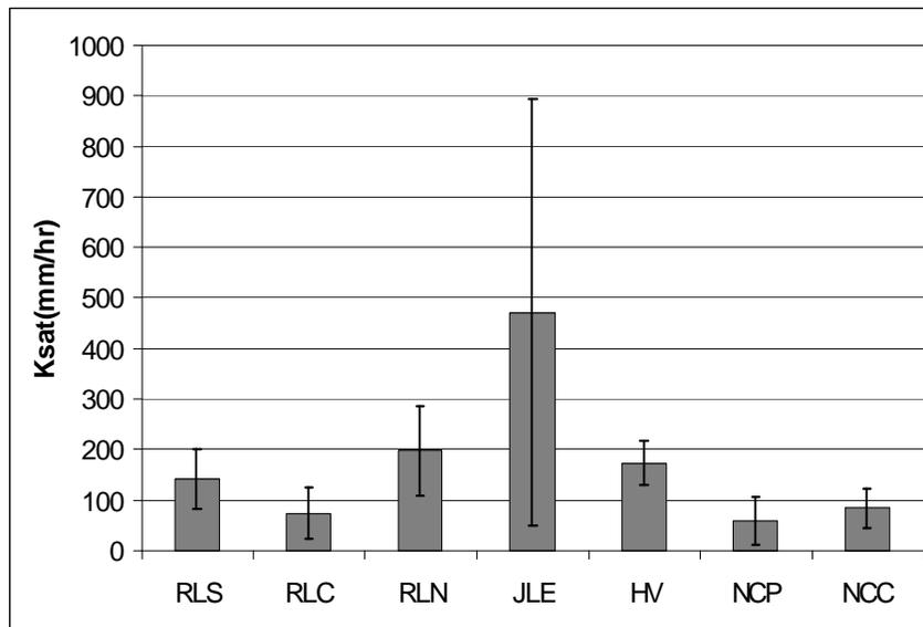
Figure 3-18. Saturated hydraulic conductivity as measured by tension infiltrometer for under canopy and interspace. Error bars represent the standard error of the mean.
