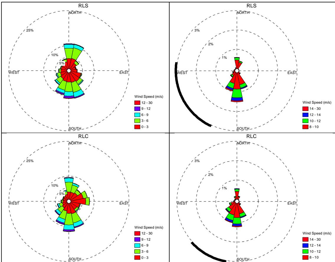
Figure 3-23. Wind roses by site for all 1-minute wind speeds (left panels) and for periods when the wind speed was greater than 8 m/s (right panels). Thick black trace in panels on the right side of the figure indicate the angle extent of nearby playa (s) as viewed from the meteorological tower at the site.
