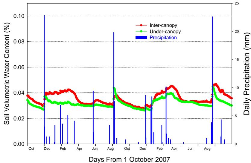
Figure 3-16. Mean soil volumetric water content for under canopy probes and inter-canopy probes.
