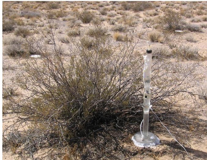
Figure 2-3. Tension infiltrometer measurement in plant under canopy.
