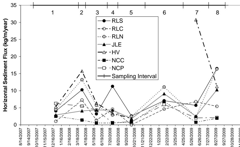
Figure 3-24. Rates of sediment transport averaged from three sediment traps at each site. Vertical lines at the top of the Figure delineate exposure periods for the sediment traps.
