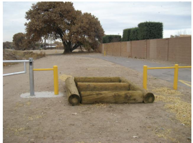
A motorized vehicle barrier that allows for equestrian passage
