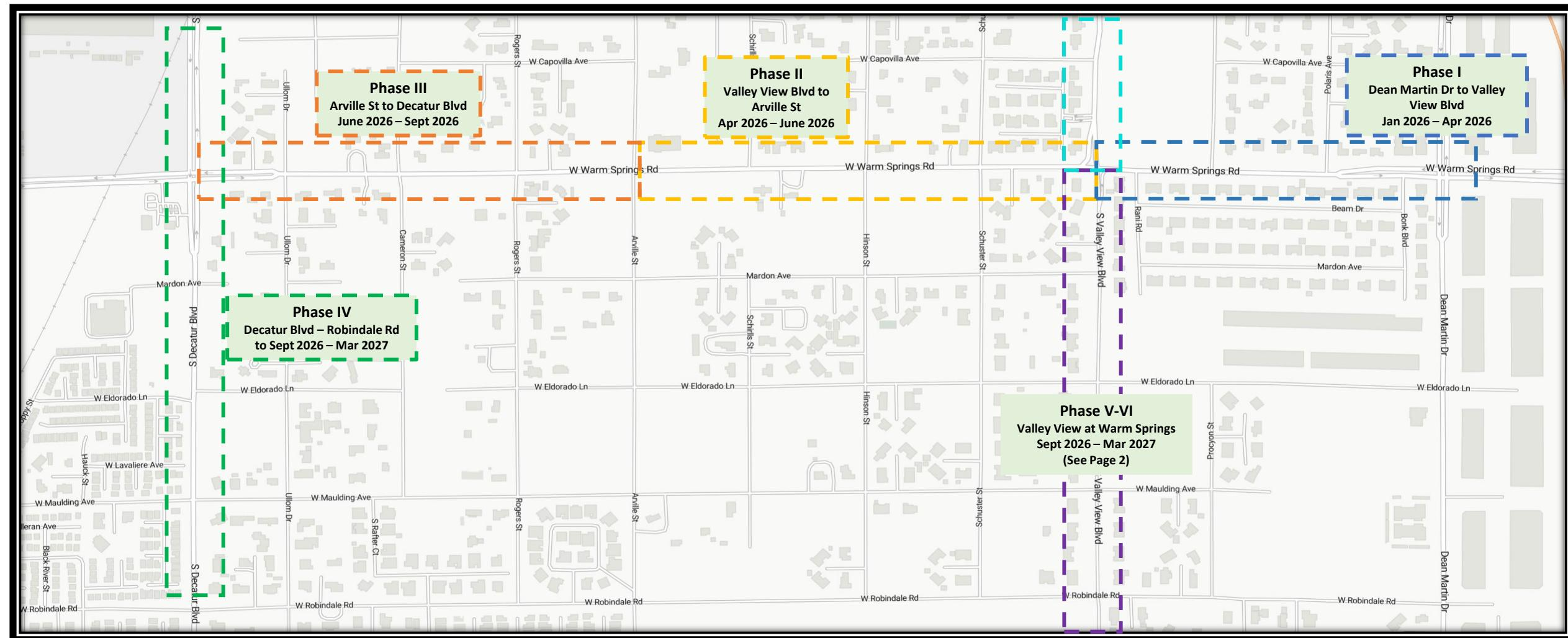
Phases I to IV work consists storm drain & sewer installation, roadway widening, concrete and asphalt sidewalk construction, ADA Ramp improvements, median island installation, pedestrian and horse crossing at Arville St, traffic signal modifications, traffic signal installation at Valley View, etc.
