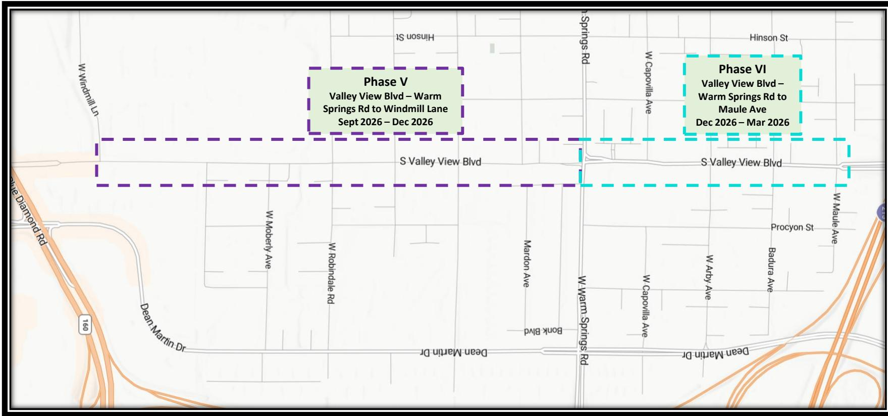
Phases V & VI work consists roadway reconstruction, striping modifications, asphalt sidewalk, storm drain modifications, etc.
