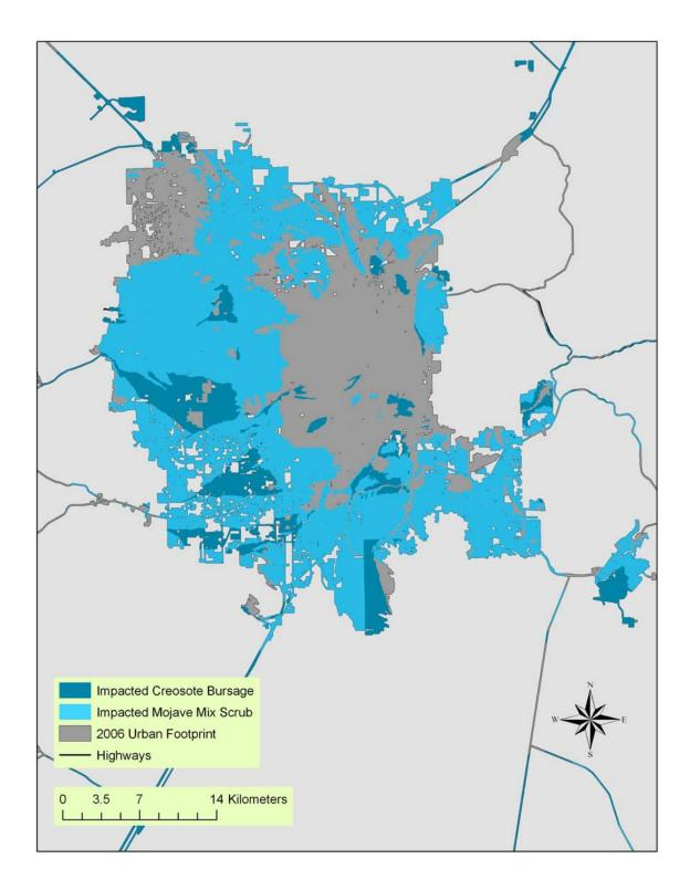
**Figure 2-17**. Estimated areas of creosote-bursage and Mojave mixed shrub lost to urbanization within Las Vegas Valley. Note the straight line between areas in the lower center of the image which is an artifact that reflects differences in the vegetation described for the soil type in different surveys.
