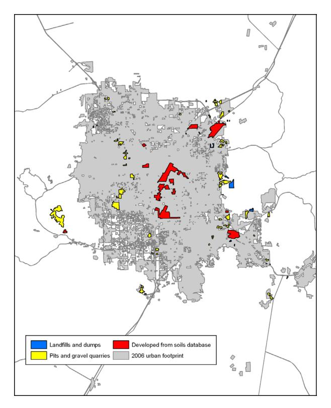
**Figure 2-16**. Map of Las Vegas Valley showing areas of high soil disturbance that could not be assessed to natural condition during the soils survey.
