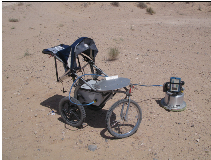
Fig. 2: Photograph of the PI-SWERL (right), with computer, battery and control box mounted on carriage (left)
