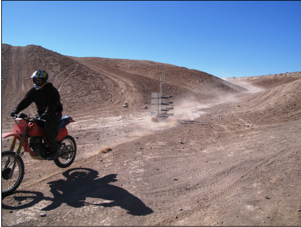
Fig. 4: Photo of the set-up of dust poles and dust traps during a dirt bike run
