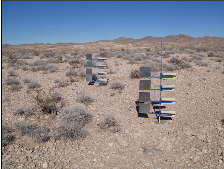
Fig. 3: Poles with BSNE dust samplers
