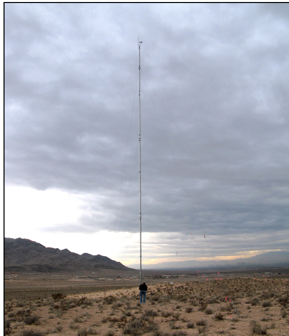
Fig. 4: 20-m wind tower with anemometer and wind vane
