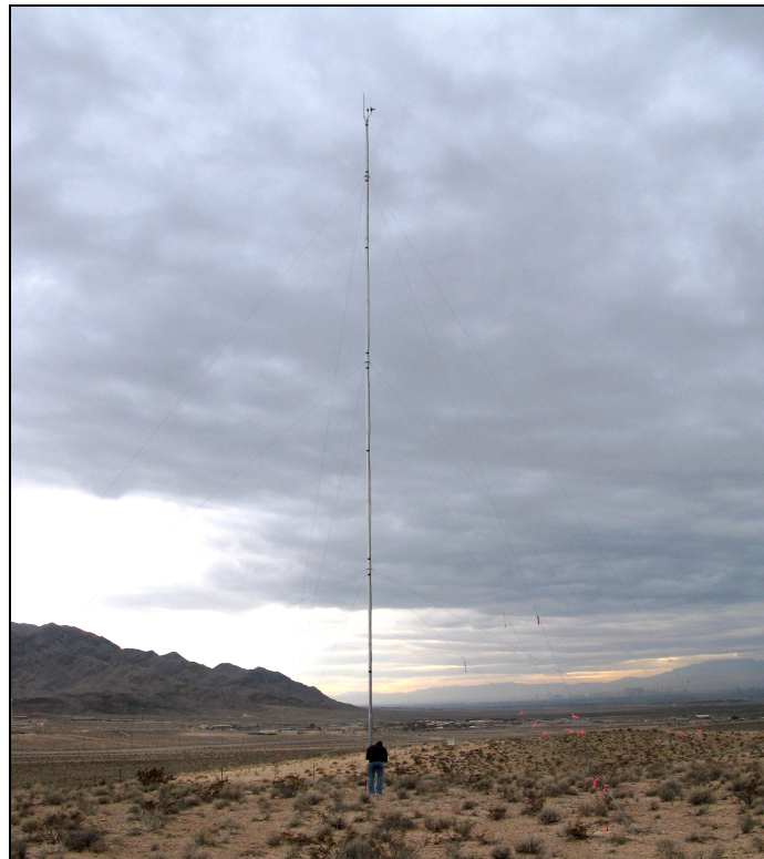
Fig. 3: 20-m wind tower with anemometer and wind vane
